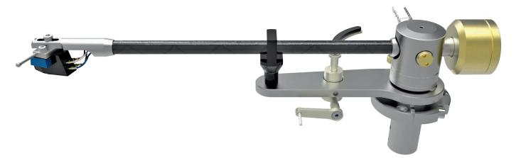
The TA-500 is a precisely manufactured precision-bearing 9 inch tone arm. The precision miniature ball bearings used are from manufacturer SKF. The bearings are added with minimal pre pressure for zero backlash to achieve a minimum friction and maximum stability. The armtube is a custom made dual carbon tube. This creates a very rigid tube but still having a high damping and resonance. The TA-500 is only available with 5 pin connector and a Audioquest 5 pin cable is supplied with the arm.
