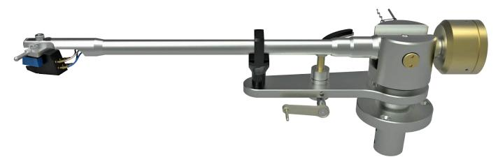
The ACOUSTIC-SIGNATURE TA-700 is a full aluminum design 9 inch tonearm. All the experience we have is built into this magic tonearm. We use bearings from a well-known Japanese Manufacturer. All bearings are closed versions to ensure no dirt or dust is affecting their lifetime. The arm tube at the TA-700 is made from a pressed aluminum bar. This bar is very rigid because of the high
