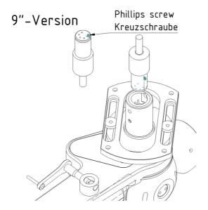
Looking from the bottom of your **TA-9000 Neo** you can see the 5 pin plug and its alignment. The connector has a small Phillips screw on its cylinder. This screw must face towards the cartridge when being inserted in the plug.
