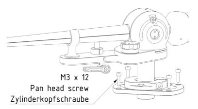
Take the provided 4x pan head screws M3x12 and insert them into the marked appropriate holes of the mounting flange (see picture above). Use the provided Allen key to tighten the screws. To get easier access to the holes, it might be helpful to turn the complete tonearm within the mounting flange so the holes are free. Or you can take out the tonearm and assemble the mounting flange first.
