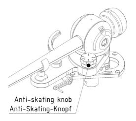
To adjust the Anti-skating use the Anti-skating adjustment knob and adjust the correct value by slowly turning the knob, starting with 0.
