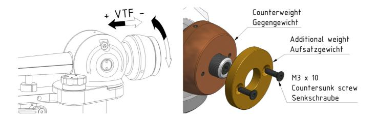
After adjusting the VTF please tighten at least one the 3 screws in the counterweight.
