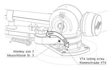
Adjust the arm height with cartridge fitted, so that the arm tube is either parallel or slightly lower at the front end.
