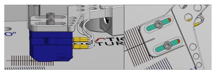
Lift down the cartridge and place the diamond tip of the cartridge on the reference point of the adjustment template and make sure that the edges of the cartridge are parallel to the marking lines printed on the template.
