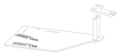
This is done by using the provided adjustment template. Take the two parts of the template and assemble it, as shown in the picture above, and place it on the platter.
