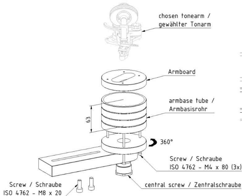
Use the delivered special wrench to handle the central screw.
