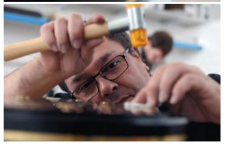
$\triangle$  Part of the assembly work is to fit the copper bars into the platter. They are fitted in one by one and then the height of each one is checked carefully. It looks very flat and level, in fact, they are hammered in by hand.
