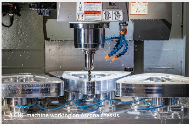
Three Ascona turntable chassis await further milling.
