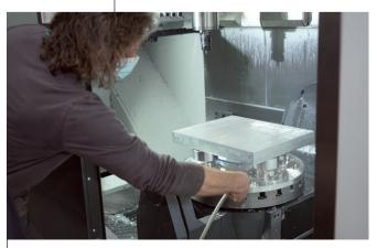
▲ CLAMPED: The workpiece is clamped at three fixing points and automatically rotated.
