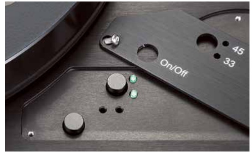
The speeds are set very precisely by the manufacturer. Corrections can be made in very fine steps via the plus/minus buttons located under the cover.
