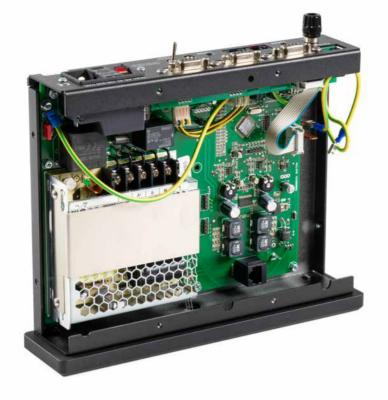
The external motor controller provides the Tornado NEO with juice and momentum. In addition, sensors provide real-time feedback regarding motor vibration. The smart electronics modulate the phase of both drives to ensure that any undesirable movements are suppressed.
