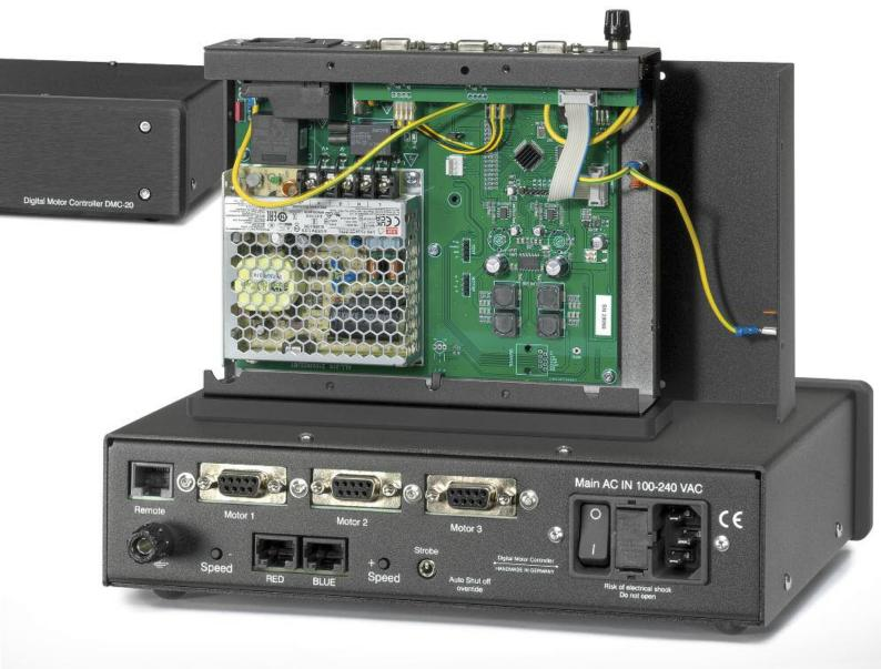
The external digital drive unit DMC-20, connected to the turntable via two Ethernet cables, ensures a permanent regulation of the phase shifts of the motor signals by means of an "Anti Vibration Control". As a result the two AC synchronous motors run with exemplary smoothness. And, in conjunction with the bearing and chassis design, the quiet operation is also transmitted to the listener
