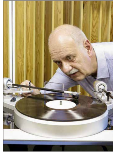
The height of the tonearms was also meticulously adjusted by means of a block with dip marks.
